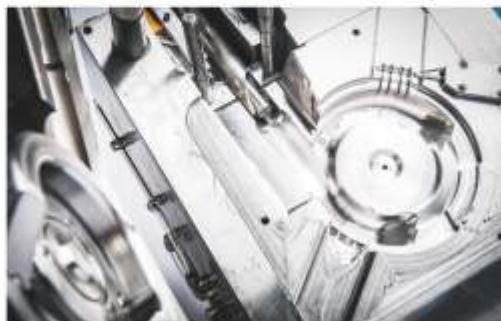
The mould manufacturing workshop is equipped with modern cad-cam assisted numerically controlled milling and electrical discharge machining equipment. It produces steel and aluminium moulds with small and medium sized multi-cavity dies.
